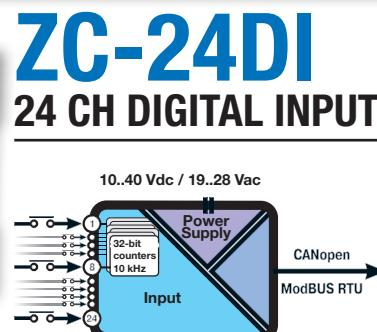
ZC-24DI is used to interface N.24 digital signals (PUSH BUTTON, LIMIT SWITCH, REMOTE, CONTROL SWITCH, RELAIS etc.) with all of control systems which are able to communicate by the protocols CANopen or ModBUS RTU (protocol selectable through dip-switch). It disposes of 32 bit counters (N.8), maximum frequency input is 10 KHz. A 3-way galvanic isolation among Power supply // input // RS485 circuits assures the integrity of your datas.
